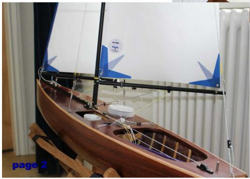
Photo left: a fine One Metre class yacht built in timber by the owner Colin Cooper. Nylet sails in white Dacron with blue standard corner patches. Photo courtesy of the owner.
